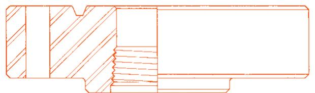
LEAD FILLED TARGET FLANGE
