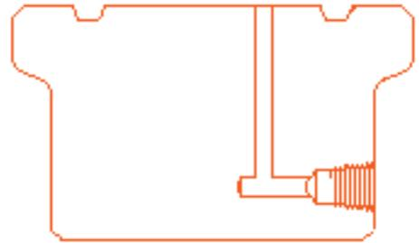
LEAD FILLED TARGET HUB FLANGE
