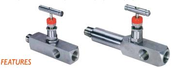
316 S.S. construction for corrosion resistance. Non rotating vee or ball tip. Extended body for insulation clearance. Scheduled 160 or heavier pipe valve inlet for strength. Optional graphoil packing available for high temperatures. Ball\*/vee tip design forms a bearing joint with the stem which eliminates rotation between ball/vee tip and seat at closure. This prevents scoring and galling up the valve seat and ensures long life in repetitive shut off service.
