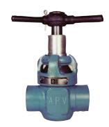
**Buna N** (nitrile) is the basic seat elastomer. It is excellent for petroleum oil an gases, fueled oils and alcohols from -10°F to +200°F. **Hypalon** is optionally offered compounded for maximum chemical resistance, particularly suited for oxidizing acids, it resists hydrocarbon oils and fuels from -10°F to +250°F. **Viton** is highly resistant to mineral acids and hydrocarbons and resists moderate concentrations of hydrogen sulphide. Serviceable from -10°F to +400°F (Not suitable for steam)
