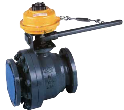
A temperature sensitive valve actuator with a self-contained energy source, for automatic valve operation in the event of a fire (fail-closed positioning).
